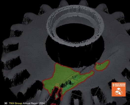
As part of LMI Technologies' commitment to innovation, the GoPxL Pro Tools series introduced the Anomaly Detector, a powerful Al-powered toolset designed to enhance 3D defect detection in production lines. This solution leverages traditional and Al-based tools within the GoPxL software framework, enabling users to train and deploy defect detection models directly on GoMax hardware without relying on additional cloud or external resources.
