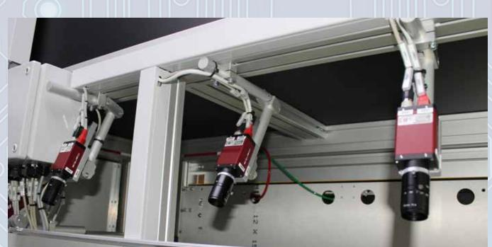
The options that a customer can choose from when buying a car seem unlimited. However, because of these different options, the production of car parts cannot be standardized, and each part must be configured separately. TKH's vision technology plays an important role in the end-of-line systems for inspection automation and quality control of door panels for cars.
